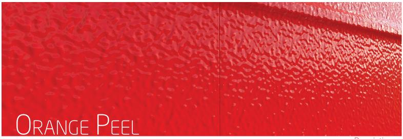
Also known as: poor flow, poor levelling, pebbling
