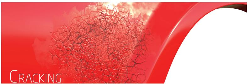
A series of deep cracks resembling mud cracks in a dry pond. Often in the form of three-legged stars and in no definite pattern, they are usually in the color coat and sometimes the undercoat as well.
